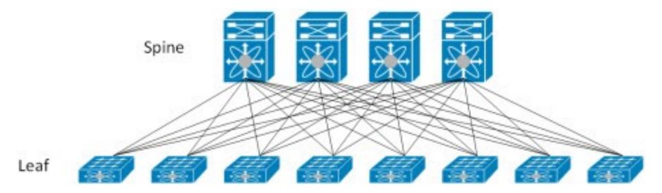
The Top of Rack (ToR) switches are the Leaf switches Each ToR is connected to multiple Core switches which represent the Spine. # of Uplinks (of each ToR) = # of Spine switches # of Downlinks (of each Spine switch) = # of Leaf switches Multiple ECMP exists for every pair of Leaf switches Support Incrementally "Scale-out" by adding more Leaf and Spine switches
