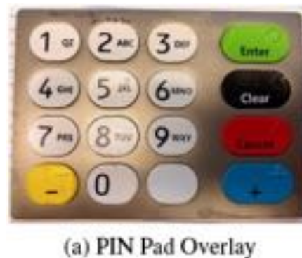
Figure 3: The front and rear of a typical overlay skimmer along with a photo of the skimmer installed on a real ATM, as captured by the NYPD. From the rear, the hardware for reading and storing the card data can be seen.
