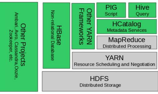
Figure 2.2 YARN adds a more general interface to run non-MapReduce jobs within the Hadoop framework
