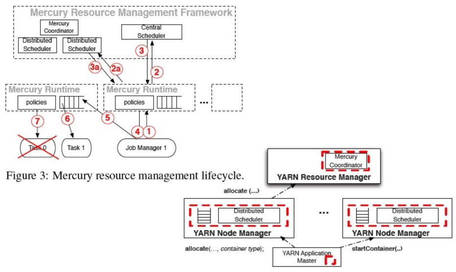
Figure 4: *Mercury implementation*: dashed boxes show Mercury modules and APIs as YARN extensions.
