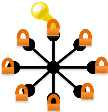
Asynchronous Execution requires heavy locking (GraphLab)
